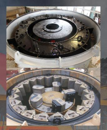
Steel-On-Steel configuration for maximum production
